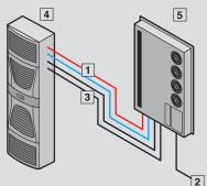
1 Flexible coolant lines inlet/return
