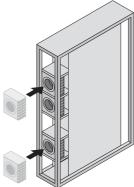
To achieve the max. cooling output of 30 kW, the customer/service needs to install two additional fan modules.
