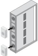
To achieve the max. cooling output, the customer/service needs to install two additional fan modules.
